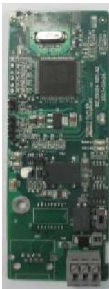
CANopen/CAN master/slave control communication card EC-TX505/511
